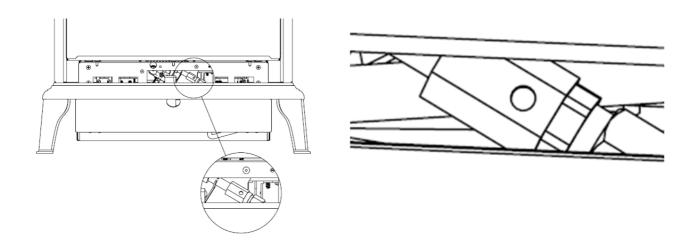
If this procedure does not resolve such a problem then the pilot assembly will need to be replaced. This must involve the installation of the same part as supplied by the manufacturer. Excessive lint build up which results in appliance operational problems is not covered by warranty. It is important to ensure this preventative maintenance is performed regularly.
