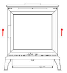
With the door frame removed, the two top glass retaining clamp can be seen.
