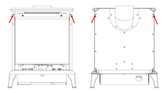
**Step 2.** Remove the four screws as shown
