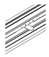
Slide the control knob to the right to the ignition symbol. After a few seconds the pilot light should light.
