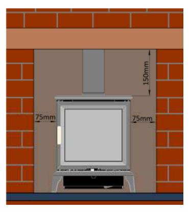
For example, shelf projection = 100mm Clearance must be 175mm (to the shelfs nearest point).
