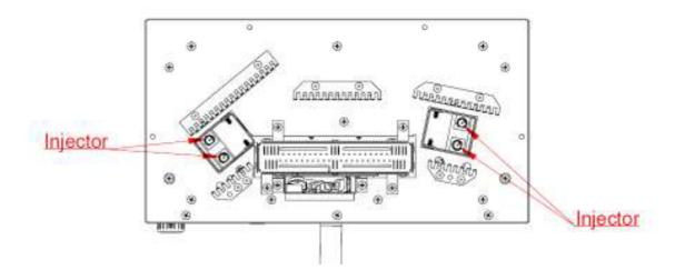
Finally remove the screw as shown below, The tee connector can be pulled out and the middle burner injector can be removed. This injector is marked 71.
