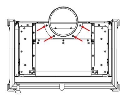
**Step 4.**Fit the ceramic gasket using the four screws provided in the rear flue kit. Then using 5 screws, attach the rear rectangular flue duct as shown.
