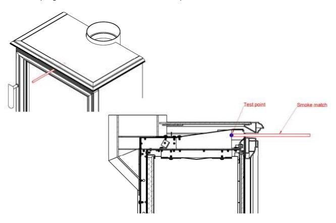
If the appliance fails the spillage test it may be necessary to install a 5" flue liner for the full length of the flue (if not already fitted). If the unit continues to fail this test, turn off the appliance and seek expert advise to expert advice.
