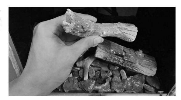
Place log F on the burner tray base at the back of the fire as shown in this picture.
