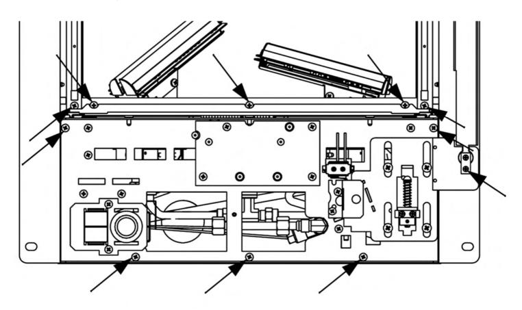
Now carefully pull the burner tray from the fire box. The burner tray is can now be serivced or repaired accordingly—see the following pages for information about removing and replacing serviceable components.
