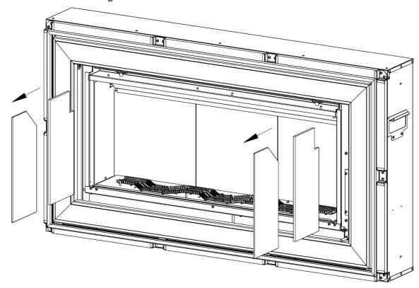
3. Lift the back glass upwards, tilt the lower edge outwards. Remove the back glass panels and the back liners.
