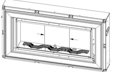
3. Finally, fit the side glass panels and side liners as shown here. Slide the liner in first and then slide the glass side panel in until it touches the rear glass panels.
