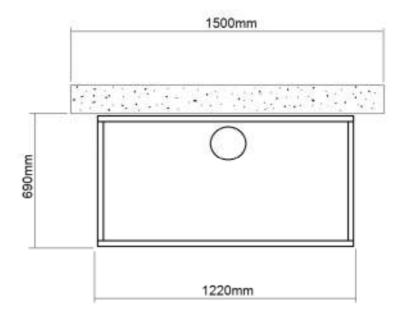
Once the lintel is secure, proceed to remove the plaster, plasterboard and inner block work to the correct dimensions.
