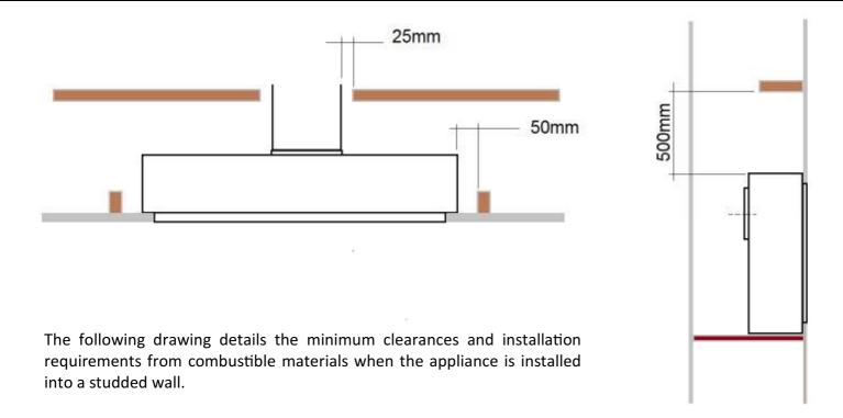
A chamber should be created for the appliance outer box installation. The chamber should he manufactured using non combustible fire-board of minimum thickness of 9mm and the clearances from combustibles (above) should be adhered to. Ensure that the chamber ventilated at the base to allow cool air to enter and ventilated at the top of the chamber to allow warm air to be exhausted into the room. This inlet/outlet vent should have a minimum open area of 100cm<sup>2</sup>.
