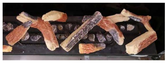
Place the ceramic bark around the ash pan base as shown below. Take care not to place any bark around the pilot burner assembly. Leave at least 5mm from any part of the pilot.
