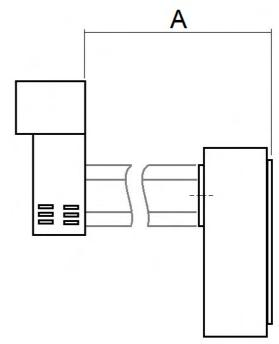
When cutting the horizontal flue section, the outer section can be cut from either side, however whichever side is reduced, the 3 securing holes should be re-drilled, using the off cut section as a guide.
